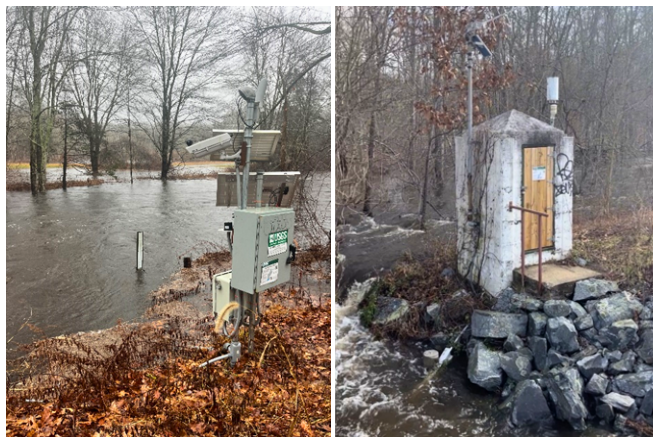
Left: Streamgage on the West Branch of the Eightmile River at North Plain, CT 01194000 Right: Streamgage on East Branch Eightmile River Near North Lyme, CT 01194500
