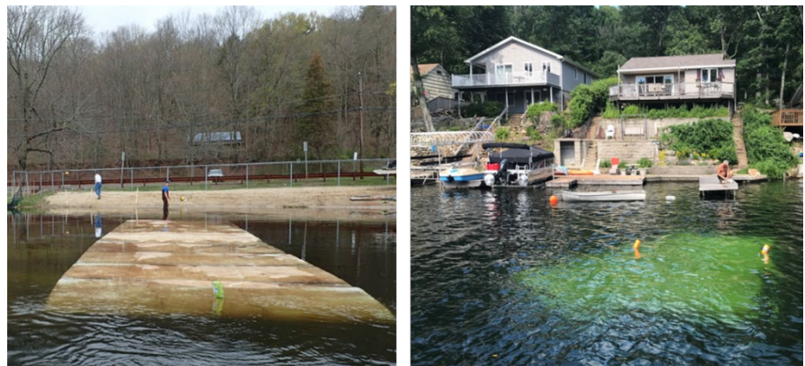
Figure 12. CAES IAPP preliminary testing of short-term benthic barriers in Lake Quonnipaug (left) and Bashan Lake (right).
