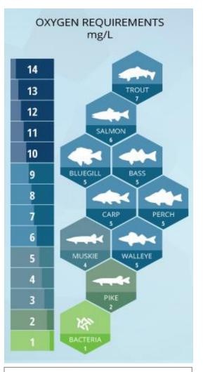
Diagram showing the Minimum dissolved oxygen requirements of freshwater fish.
