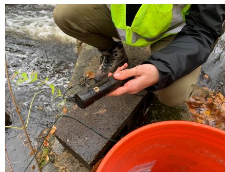
Using conductivity loggers to measure dissolved inorganic solids, such as chloride, in local streams
